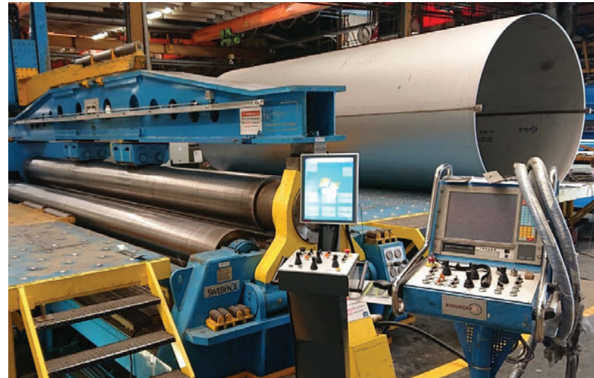
A Roundo PASS plate bending roll is upgraded to the latest SweBend SEVENX Controller
