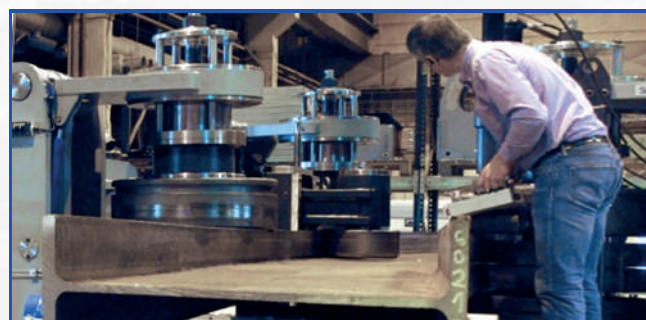
Rolling a HEA800 in a variable geometry Section Bending machine
