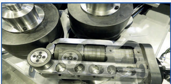
On models SB3S-XXX it is possible to have the guide rolls adjustable also in the plane of rolling. (traverse)
