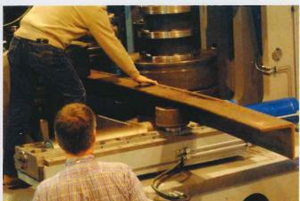
Thanks to the unique possibility to adapt the geometry geometry for each type of section the VSB can roll angle bar as easily as large H-beams.
