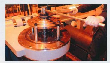
Machine design is made with supported shafts which adds numerous advantages, such as reduced shaft sizes, higher accuracy and less costly tooling. Normally the disadvantage would be the tooling adjustment but not here — **SweBend** has managed to solve this problem in a fantastic way, allowing quick adjustment of the bending rolls when required to set up the next job. And in bending business it is important to be efficient and keep the setup time as low as possible.
