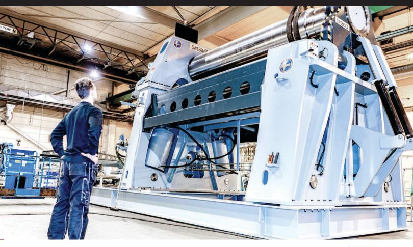
As standard, all SweBend bending rolls are equipped with basic wired or wireless controls and require manual operation by a skilled operator.
