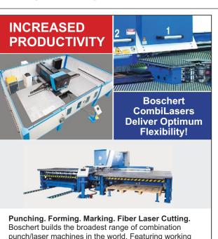
Boschert builds the broadest range of combination punch/laser machines in the world. Featuring working ranges from 30" x 80" to 60" x 120" plus repositioning. One, two or three punching heads or fully automatic tool changer. With full rotation, multi-tool, vertically moveable dies for deep forms and punching force to 50 tons.
