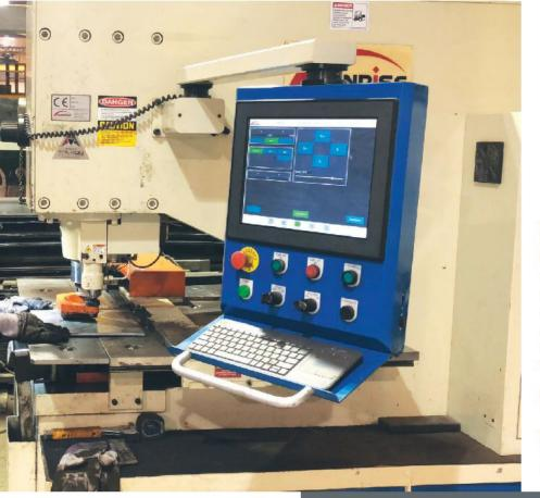
uted exclusively by Trilogy Machinery. Rollers make it easy for operators to move heavy material across the punch. Its hydraulic hold-downs prevent material slippage and allow SteelMart to produce accurate, consistent holes. The Sunrise punch is equipped with a CNC backgauge that can be programmed to run multiple parts quickly.
