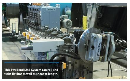
manufacturing line trims the flat ends and rolls a perfect part without the need for a secondary operation. These cells also lend themselves to a SweBend roll bender equipped with a CNC or PLC for automation. We have customers integrating these systems with robots and other advanced automation."
