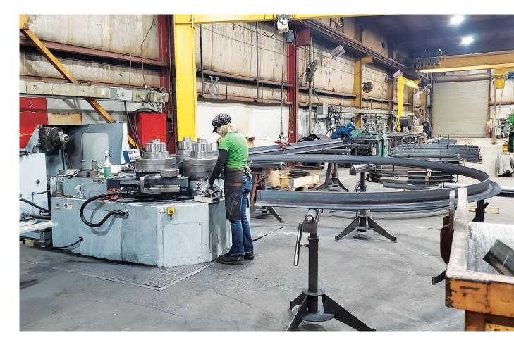
Trilogy customized the SweBend section benders with faster rolling speeds and more bending power.
