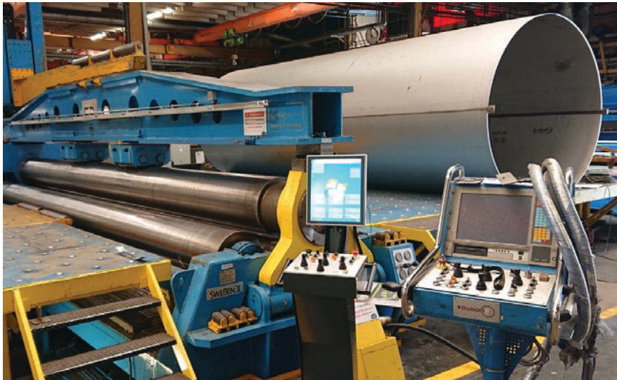
A Roundo PASS plate bending roll is upgraded to the latest SweBend SEVENX Controller
