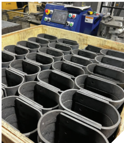
U-shaped parts are a good fit for a horizontal bending machine's forming action.
