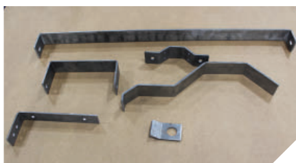
Brackets of all sizes can be quickly formed on a horizontal bending machine.
