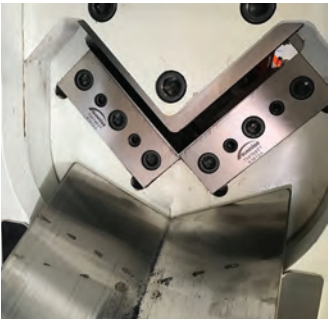
No slug shear with multi-sided blades, adjustable blade gap
